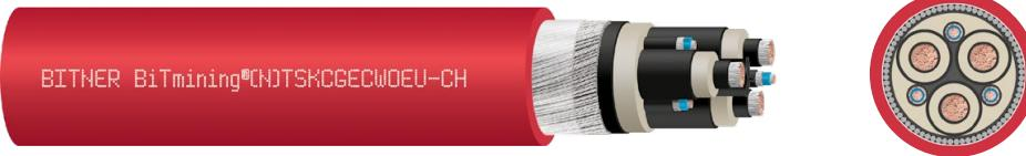
**Application:** Flexible power supply cable for use in underground mining facilities for mobile machines like coal cutters etc. Designed for use in cable chains trailed behind the machines. Chains have protective function and absorb the tensile forces occurring during operation.
