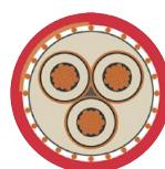
**Application:** Cables are designed for connection between frequency converters and medium voltage motors. They are suitable for installation inside buildings, in dry and moist rooms.
