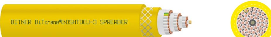
**Application:** Reeling cable for vertical drum-spreader systems for energy and data transfer to "headblock" e.g. on Ship-to-Shore container cranes with high mechanical stress. Depending on installation situation monospiral or cylindrical reels are used. Typical hoisting speed on Super Panamax / Megamax STS gantry crane types: up to 180 m/min.
