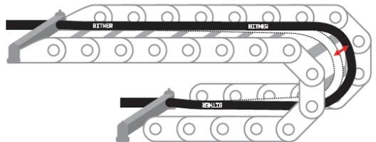
There must be no cable tensile forces over the entire drag chain.
