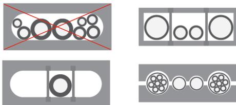
**Note:** incorrect distribution or cables fastening can result in unwanted cable movement against each other that can cause their blocking in the tray, deformation of cable assembly, insulation or core damage. Moreover, it can shift the centre of gravity of the installed cables what can in turn change operating path and cause mechanical damage of the drag tray.
